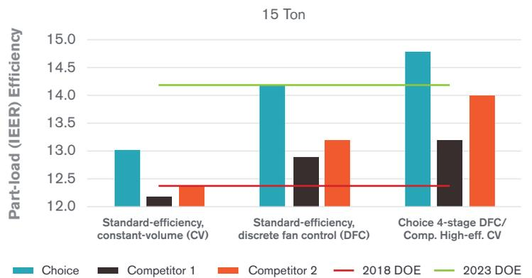
Standard-efficiency TempMaster® Omni™ Choice rooftop units with the optional 4-stage IntelliSpeed™ fan control have better efficiency than even the "high-efficiency" models from competitors.
